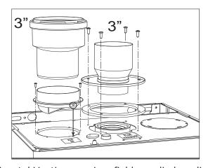
Horizontal Venting requires field supplied appliance adapter for the boiler flue outlet. Boiler is provided with a 3" vent connection, 3" x 4" increaser must be field sourced for chimney application. This does not mean that the connection to the chimney will always be 4".
